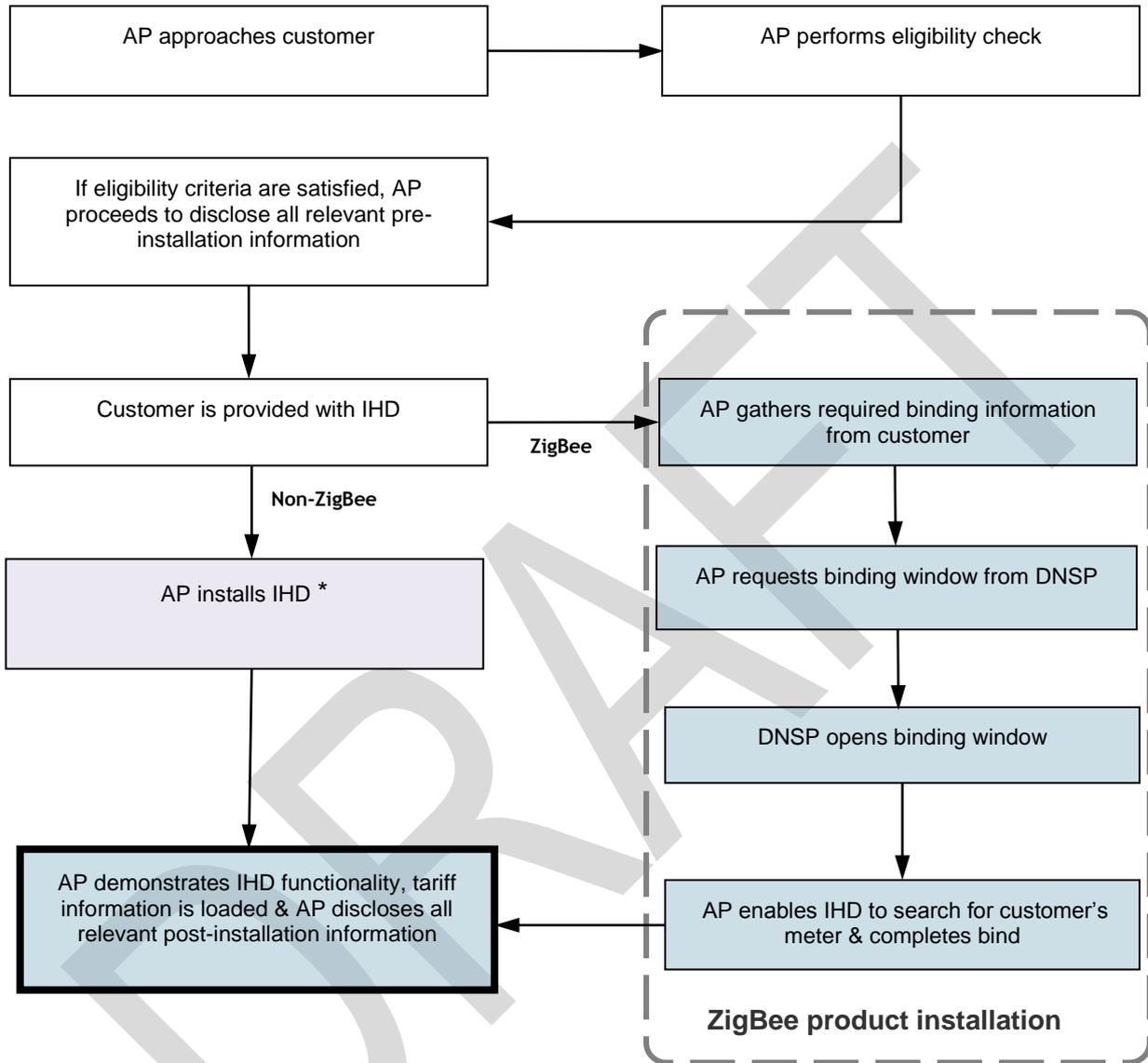
\*Non-ZigBee IHD units are required to be physically installed on premises by the AP. If the device is a clamp-on-type, it must be installed by a qualified and licensed electrician.
